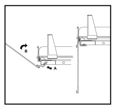
2. Starting from one end, pull gripper portion of flip sign onto metal flange (A) while rotating sign up (B). Continue until sign is securely attached.
