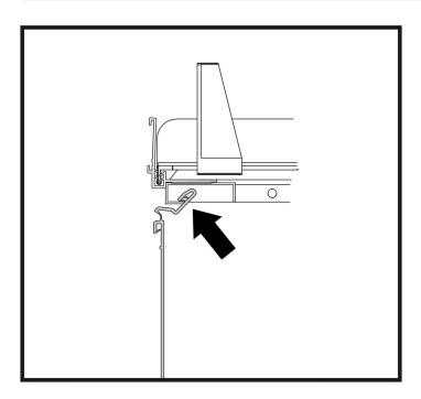
**1.** Hook sign channel onto metal flange located on bottom front of shelf.
