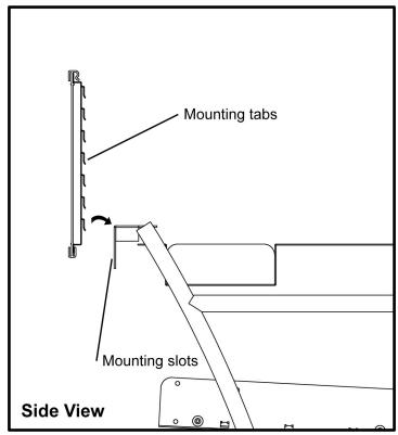
Hang the sign channel mounting brackets on the metal fixture by engaging the selected sign channel mounting tabs in the mounting slots located on the metal fixture. Push down on channel to secure mounting tabs in mounting slots. **Note:**Normal setting is in the highest position.
